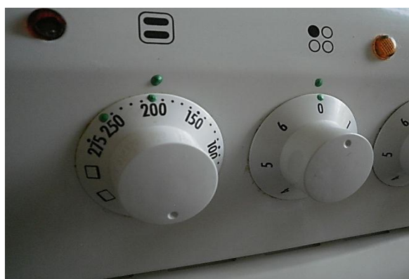
Figure 15: This image shows the control panel of a kitchen oven. The turn knob is marked so that a reference point can be determined by touch. It is important to establish a reference point in relation to the marking, a starting point needs to be marked on the device to which the marked button is adjusted.
